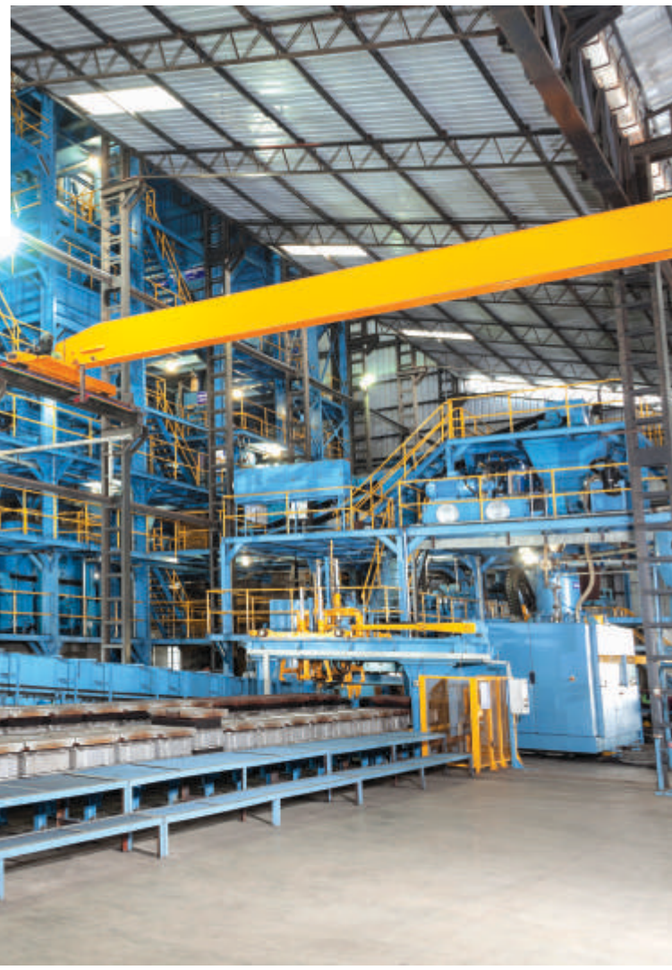
▼ Sand plant of capacity 40MT/hr.
